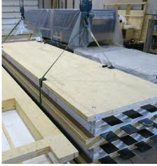
The maximum panel size is 3.5m x 6m. These dimensions are optimized for highway transportation. In the image above, CLIPs with foundation connections pre-installed are sequenced, stacked and ready for protective wrapping to be applied prior to loading and shipping to the site for rapid assembly.
