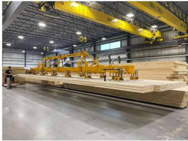
Figure 1 Element5 CLT manufacturing line [Photo courtesy: Element5]
